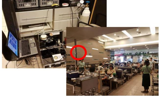
Fig. 1 Portable electronic nose for odor level monitoring in the restaurant.
