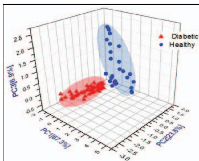
Figure 4. Results of principal component analysis of a chemiresistive sensor arrays for specimen urine odor classification.
