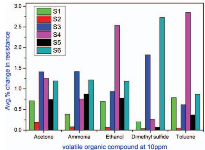
Figure 2. Electrical resistance changes of six chemiresistive sensors on exposure to (a) acetone, (b) ammonia, (c) ethanol, (d) dimethyl sulfide, and (e) toluene vapours at 10 ppm concentration.
