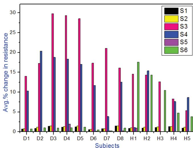
Figure 3. Sensitivity factors of the six chemiresistive sensors responding to volatile urinary components from type II diabetes patient (D1-D8) and healthy controls (H1-H5).
