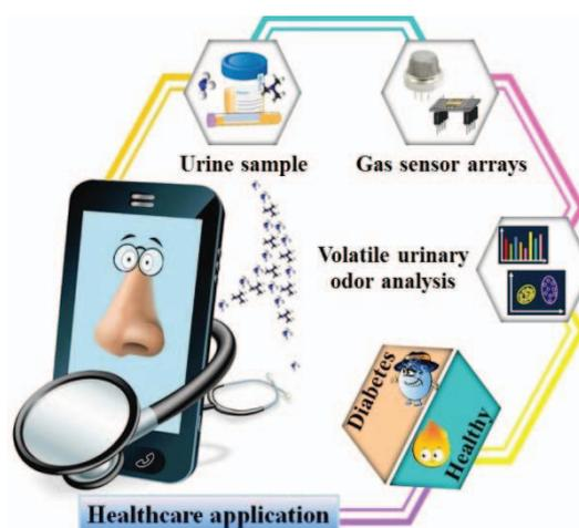
Figure 1. Schematic diagram shows the operating procedures for chemiresistive sensor system for urine odor screening in type 2 diabetes.
